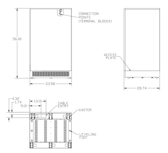
Figure 11 – "B" Battery Cabinet Drawing for 24/36kVA Ratings
